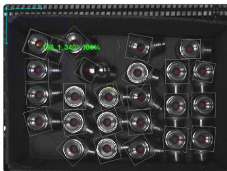
3D Bin picking in a box of valves. Scorpion sends the valve positions to the robot.
